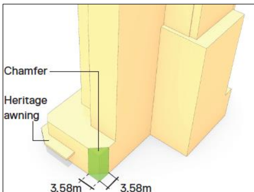
Figure 1: Podium Chamfer (Source: Grimshaw)
