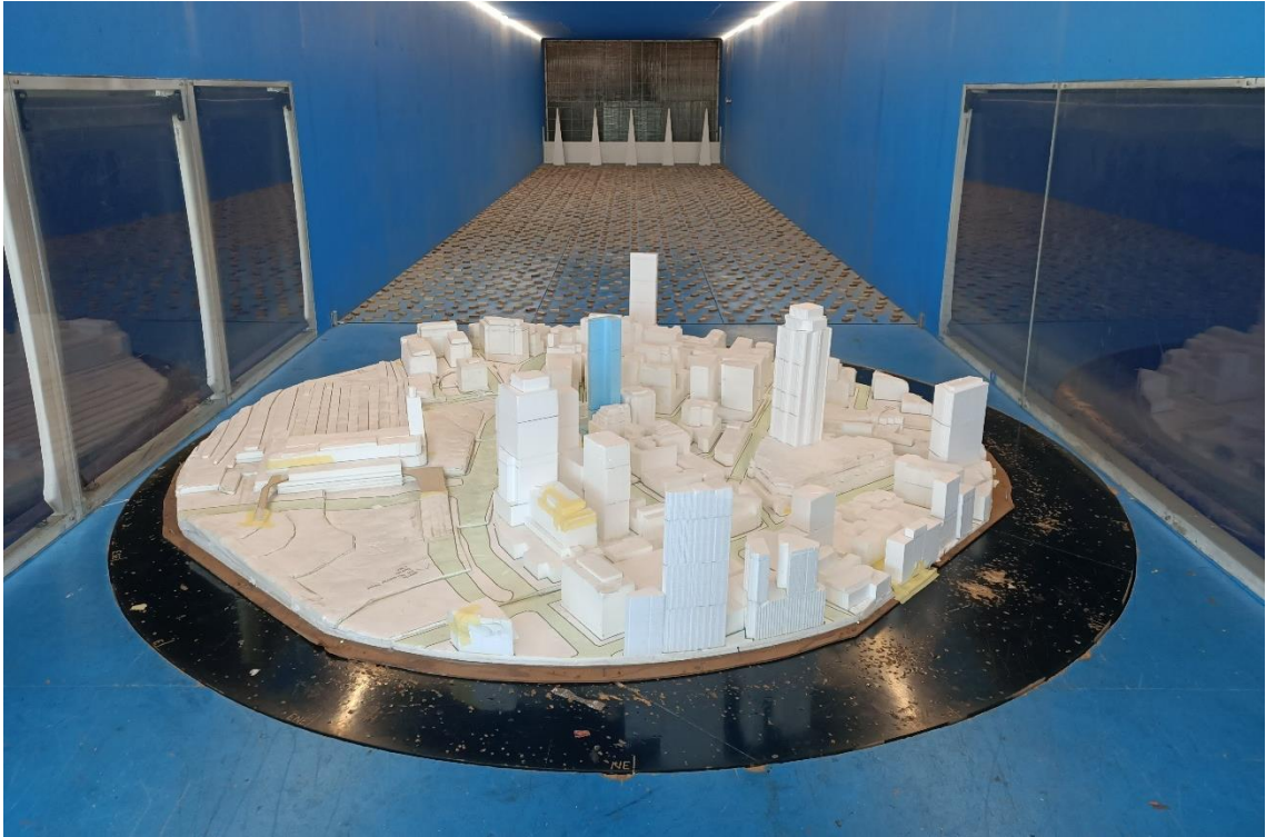
Figure 1b: Photograph of the Wind Tunnel Model (Base Case, view from the north-east)
