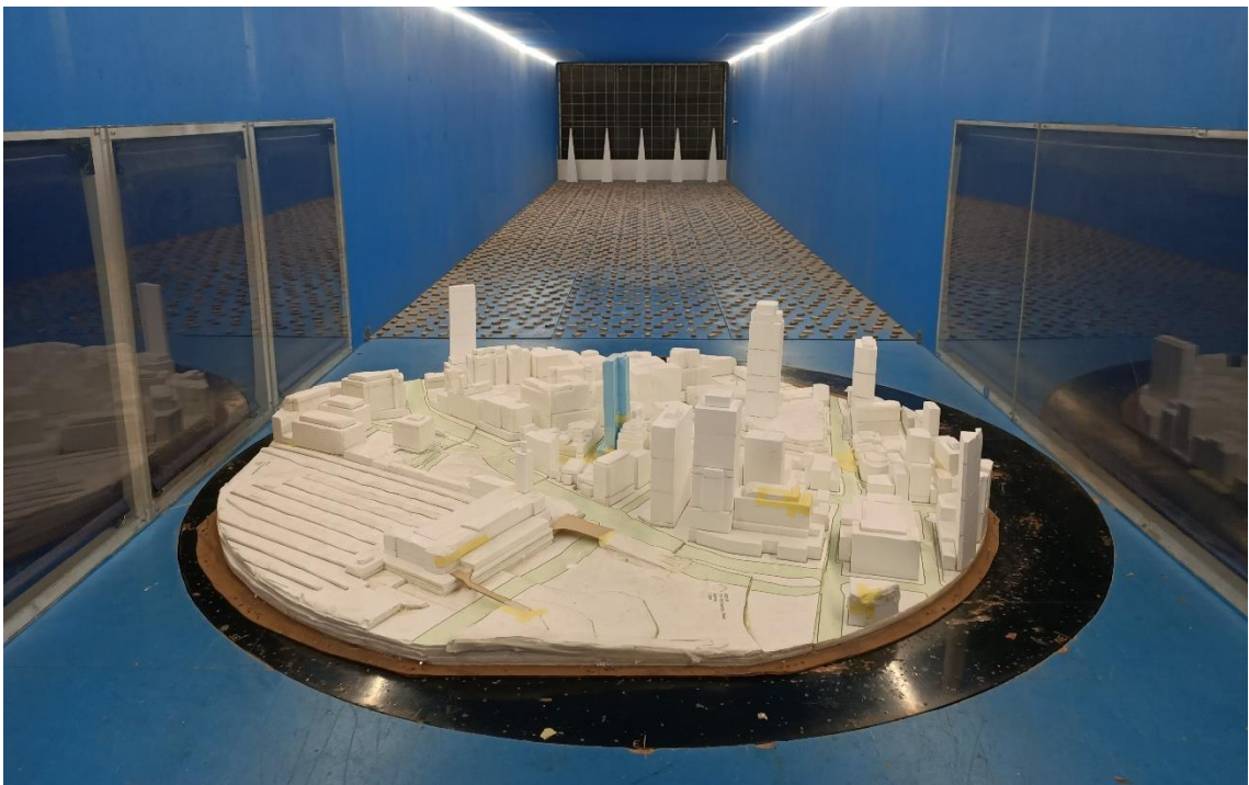
Figure 1h: Photograph of the Wind Tunnel Model (Proposed Case, view from the east)
